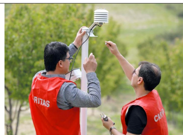
Installation of low-cost weather station in Tajikistan.
