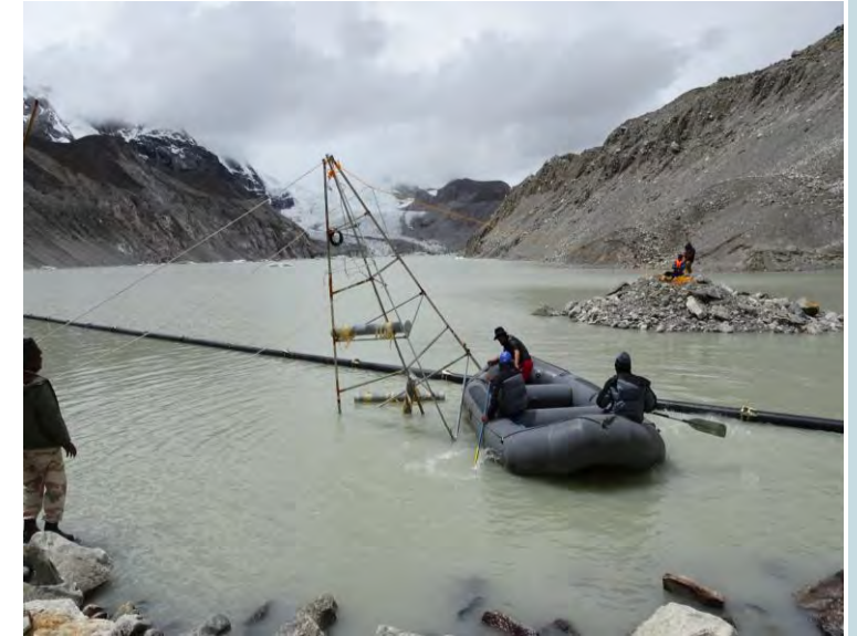
Water level monitoring sensor being installed at South Lhonak Glacial Lake
